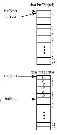
What would happen next is the process to empty the buffer would start up, and the first few characters would be sent out. The bufStart index would start to move such that it begins to catch up to bufEnd. If nothing is printed, the bufStart pointer eventually catches up with bufEnd. When the two are equal, the print buffer is empty.
